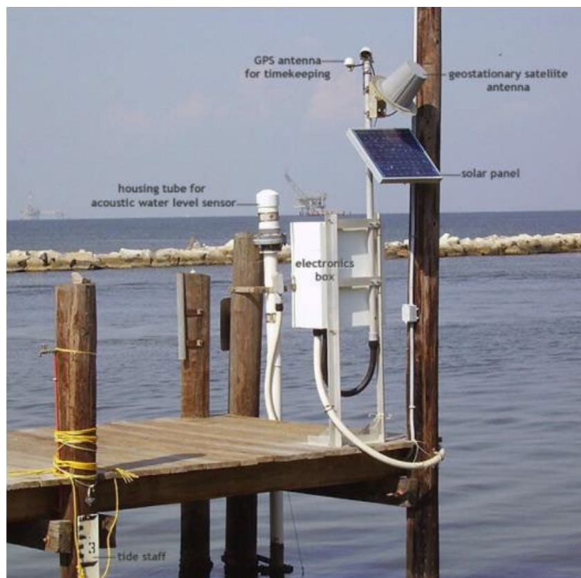
Figure 3.5. The figure shows an example of fixed-point gauge station by a NOAA water level monitoring station on Dauphin Island, Alabama ( www.climate.gov/news-features/climate-tech/reading-between-tides-200-years-measuring-global-sea-level ).
